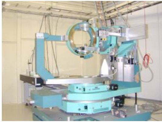
Fig.1. The eight-axis diffractometer in experimental hutch
