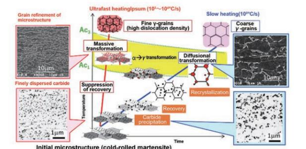
Fig. 2 Structural changes during ultrafast heating.
