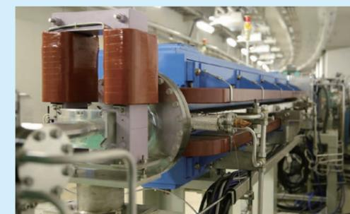
Other than standard in-vacuum type, in-vacuum revolver undulator, invacuum figure-8 undulator, twin helical undulator, tandem vertical undulator, elliptical wiggler, and others are installed in SPring-8. These insertion devices generate various polarized radiation.
