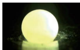
**Fig. 1** Oxide melt levitated at high temperature (by courtesy of Atsunobu Masuno, The University of Tokyo)
