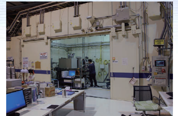
Experimental Station in Experimental Hall Synchrotron radiation from a bending magnet or an insertion device is modified with optics and led to the experimental station. A sample is studied by measuring X-ray scattering / diffraction, X-ray absorption, fluorescence X-rays, secondary electrons, and so on.
