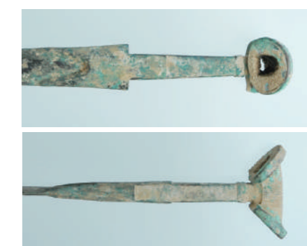
Fig. 1 "Ear pommel sword" considered to be world's oldest example of insert casting.
