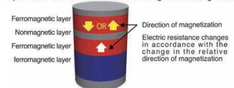
Fig. 1 Spin valve thin film in spintronic devices such as hard disk drive
