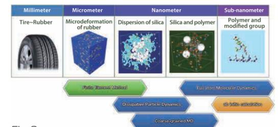
Fig. 2 Multiscale simulation enabling analysis over a wide range of spatial scales
