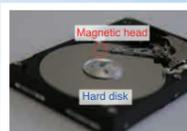
Spin valve film: an element used in magnetic reading head
