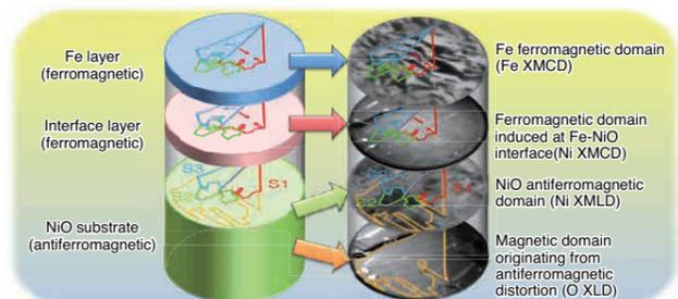
(Top) Schematic of magnetic domain observed by PEEM. (Bottom) Results of observation of magnetic domain in antiferromagnetic substrate and in Fe surface and interface of Fe/NiO(100). The arrows indicate the directions of magnetization (spins) in magnetic domains
