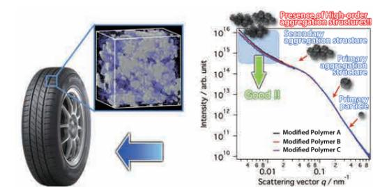
Fig. 1 One-dimensional scattering profile obtained by superimposing 2D-USAXS and 2D-SAXS data
