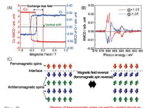
Fig. 2 (A) Element-specific magnetization curves of ferromagnetic Co spins and antiferromagnetic Cr spins obtained by XMCD measurement. (B) XMCD spectra of Cr and (C) expected spin structure at the interface
