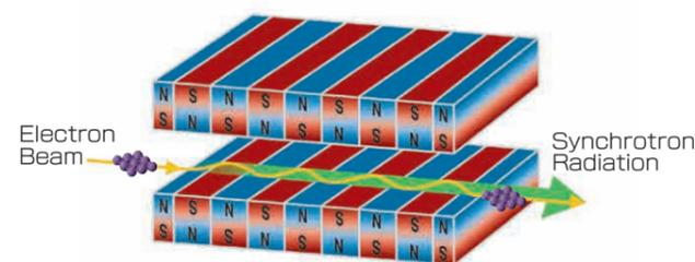
▲Synchrotron radiation produced at an undulator
