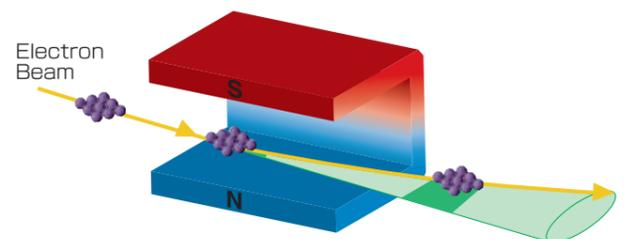
▲Synchrotron radiation produced at a bending magnet
