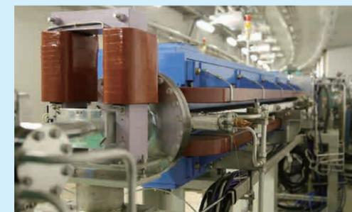
A bending magnet is a part of the storage ring that bends the electron orbit and emits white X-rays with the characteristic photon energy of 28.9 keV.
