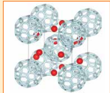
" Crystal structure of high-Tc superconducting fulleride C 33 C 60 " ( Durham Univ. / Univ. of Liverpool )
