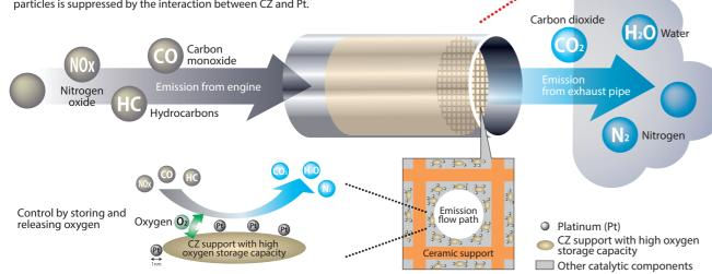
**Relationship between structure of CZ support** and oxygen storage/release performance
