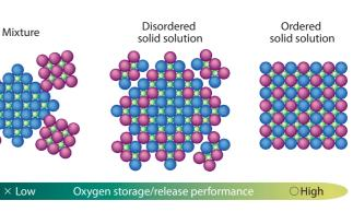
When Pt/CZ catalysts are exposed to high-temperature gas, Pt-O-Ce bonds are formed by the interaction between Pt and CZ, preventing the aggregation of Pt particles. Under normal conditions, catalytic reactions are induced when the bonds break, resulting in the lasting activity of the catalysts.
