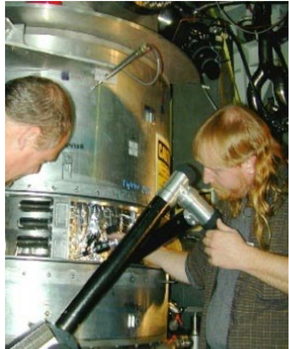
Fig. 2 Alignment of Cryo target using FaroArm
