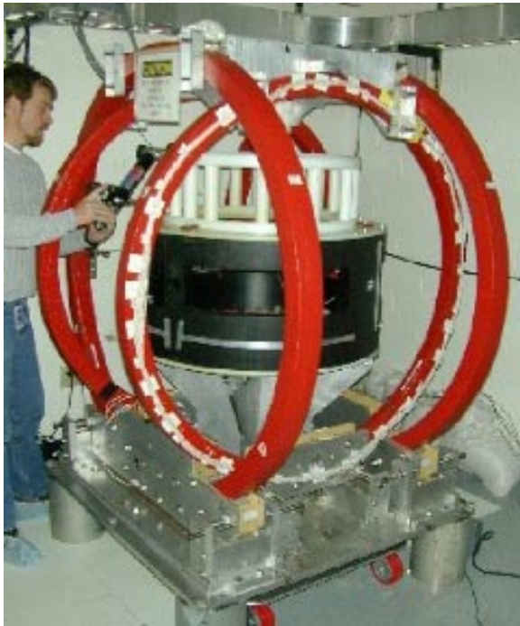
Fig.1 FaroArm Fiducialization of Hall A polarized target.
