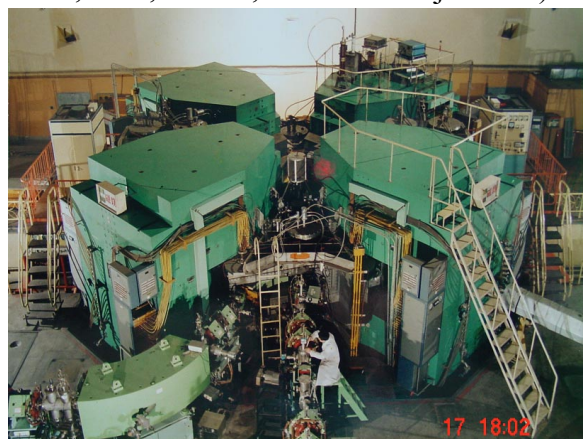
The original point of HIRFL-CSR global control Fig. 2. Separate Sector Cyclotron (SSC)
