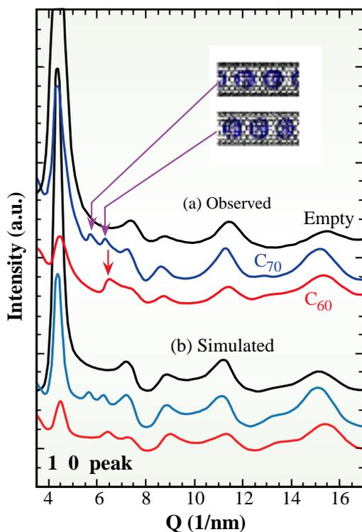
Fig. 2. The observed and simulated XRD patterns for empty SWNTs,  $C_{60}$ - and  $C_{70}$ -peapods.
