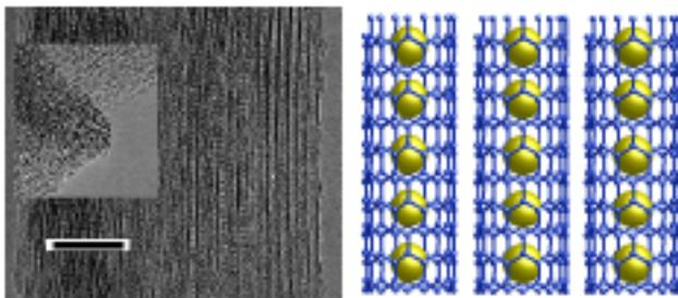
Fig. 1. The TEM image of  $C_{70}$ -peapods (left) and a schematic view of peapods (right). The scale is 10 nm. The inset shows a cross section of a bundle.
