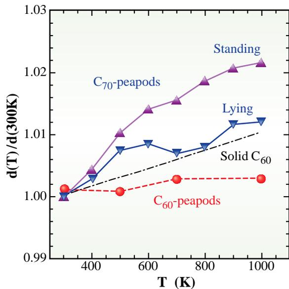
Fig. 3. Intermolecular distance of  $C_{60}$ - and  $C_{70}$ -peapods, normalized at 300 K, as a function of temperature.
