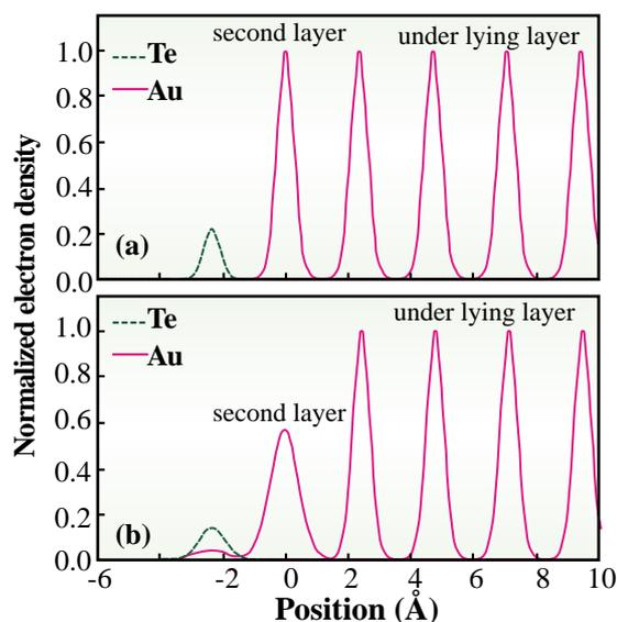
Fig. 3. Normalized electron density profile normal to the surface for fit to the observed specular X-ray reflectivity. A negative value of position means that a layer is out of the ideally terminated Au surface. (a) Model for the top layer consisting of 0.33 ML Te. (b) Model for the top layer consisting of 0.33 ML Te and 0.08 ML Au, and the second layer consisting of 0.92 ML Au.
