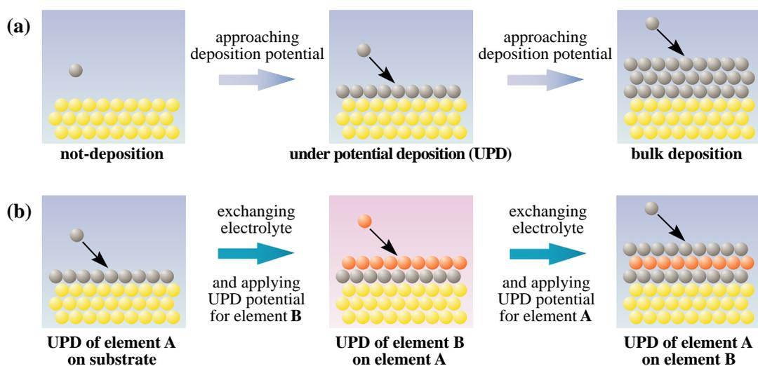
Fig. 1. Schematic illustrations of (a) underpotential deposition (UPD) and (b) electrochemical atomic layer epitaxy (ECALE).
