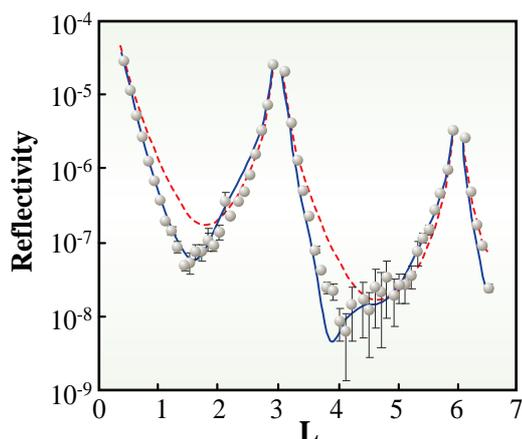
Fig. 2. Specular X-ray reflectivity from the Te UPD layer on the Au(111) substrate. The data collection was performed between 39 to 59 hours after the UPD potential had been applied. The dashed red line shows the reflectivity expected for a Te layer immediately above the Au(111) substrate. The solid blue line shows the reflectivity expected for the top layer consisting of the UPD Te atoms and Au atoms which diffuse from the Au(111) substrate.
