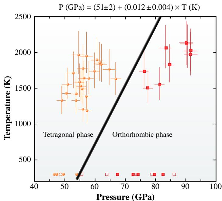
Fig. 2. The experimental results and a phase boundary determined by in situ observation. The solid circles and squares represent conditions where the tetragonal and orthorhombic phases were stable [9]. The open symbols represent data from Andrault *et al.* [3]. The solid line is the inferred phase boundary between the tetragonal and orthorhombic phases in silicon dioxide.
