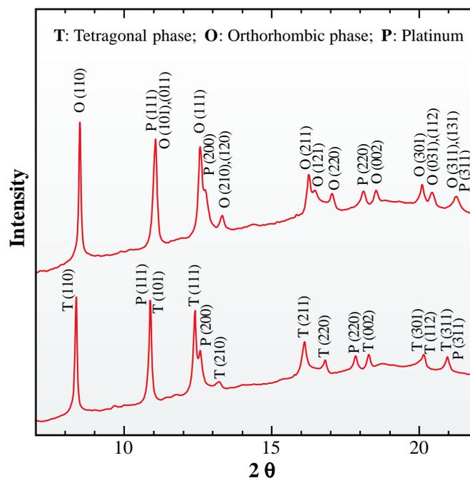
Fig. 1. X-ray diffraction patterns for silicon dioxide phases using angle-dispersive technique with DAC experiments.
