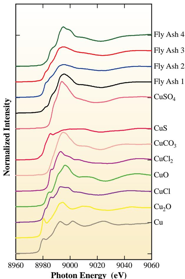
Fig. 1. Cu K-edge XANES spectra in fly ash and reference materials.
