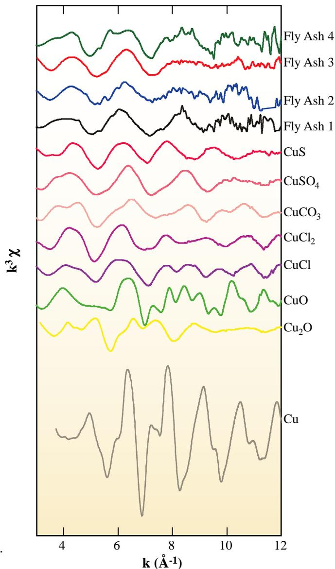
Fig. 2. EXAFS spectra of Cu in fly ash and reference materials.
