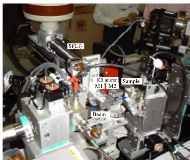
Fig. 1. Experimental setup for the X-ray microprobe.
