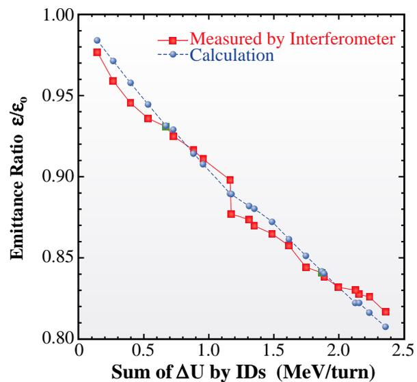
Fig. 2. Calculated emittance reduction rate against radiation loss by IDs as compared to measured value by interferometer, where  $\epsilon$ : with IDs and  $\epsilon_0$ : without IDs.
