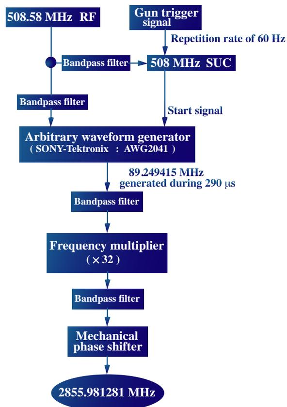
Fig. 6. Block diagram of the new synchronization method between the 508.58 MHz and 2856 MHz RFs.
