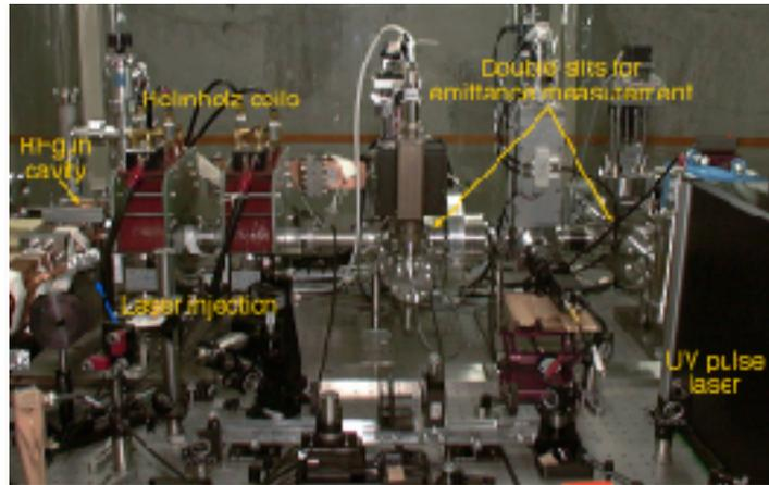
Fig. 5. RF-gun experimental setup on an optical bench.
