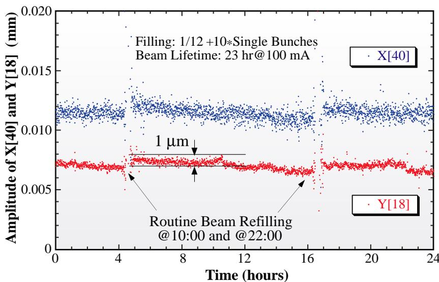
Before these improvements, the amplitude changes were about 5  $\mu$ m for horizontal and about 3  $\mu$ m for vertical. To achieve further orbit stability of sub-micron, a task force for orbit stability was organized and has been conducting overall improvement activities from a multilateral point of view.
