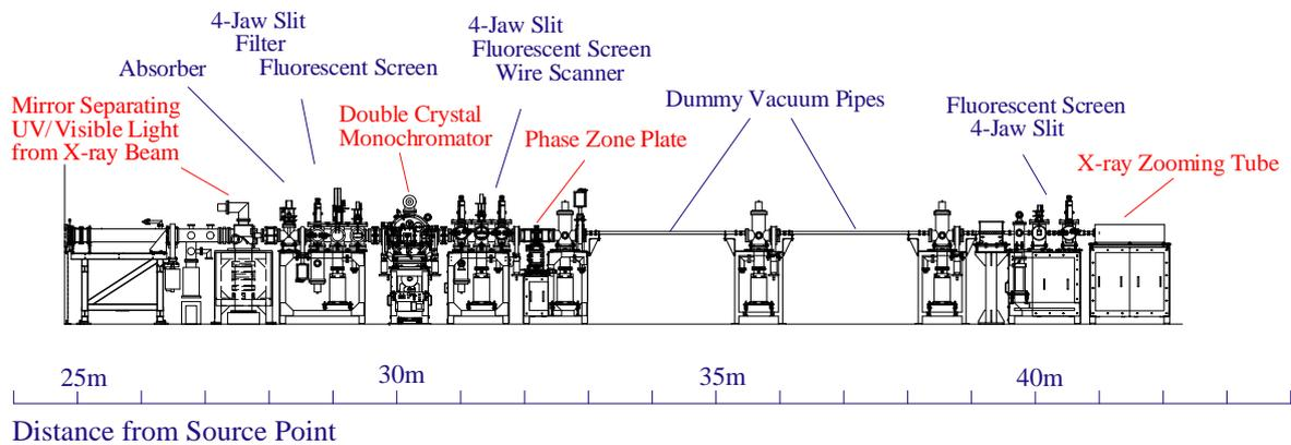
*Fig. 3. X-ray transport line of accelerator beam diagnostics beamline #1.*
