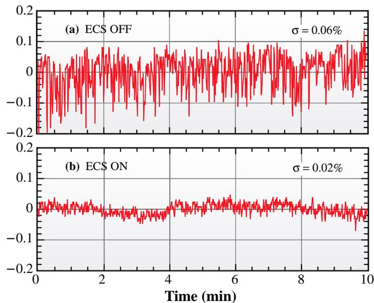
Fig. 4. ECS reduced the energy fluctuations of 1 ns beams at 1.9 nC.
