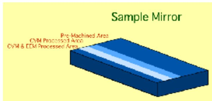
*Fig. 2. Sample mirror. A (001) surface of Si (50 mm × 100 mm) was firstly finished with a conventional polishing technique (Pre-Machined Area). A striped area was refined by a CVM technique, and a part of this was further refined by an EEM technique.*
