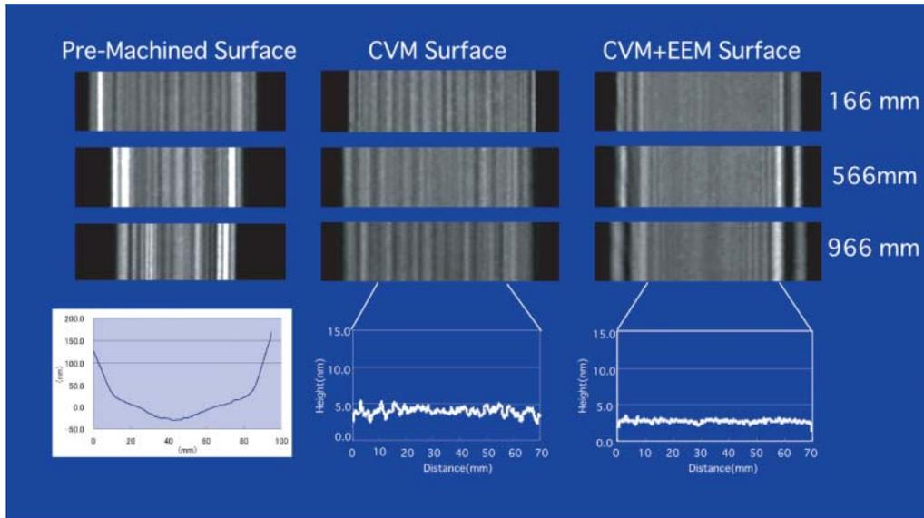
Fig. 3. Images of reflected beams from conventionally polished (designated as Pre-Machined) area, CVM finished area and a CVM+EEM finished area recorded at 166 mm, 566 mm and 966 mm from the center of mirror. Corresponding surface profiles measured with an optical interferometer are shown. Glancing angle of 1.2 mrad at 15 keV X-rays.
