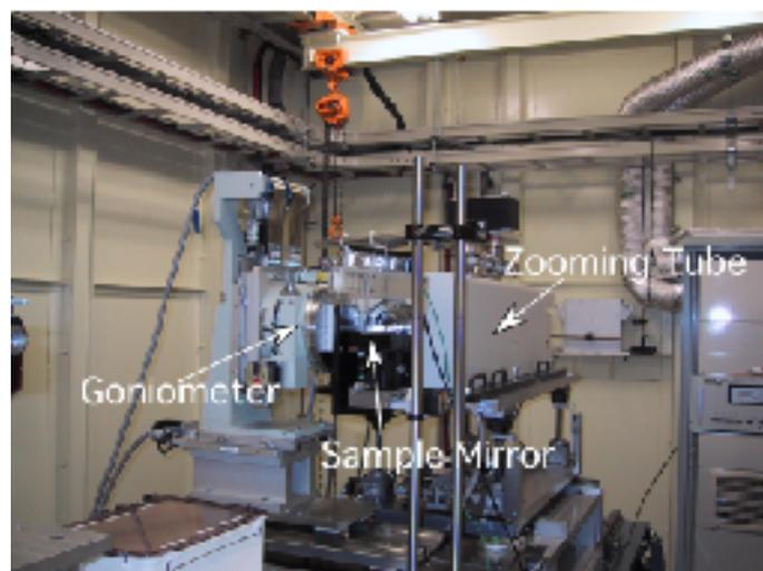
*Fig. 1. A mirror characterization setup constructed at the 1-km endstation of BL29XUL.*
