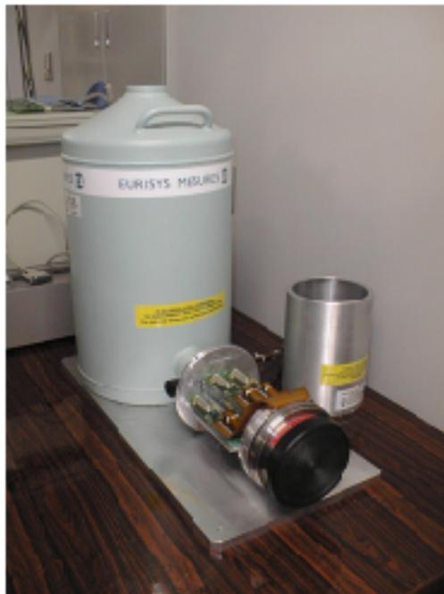
*Fig. 1. 128-channel microstrip Germanium detector with four 32-parallel-input front-end hybrid boards mounted.*
