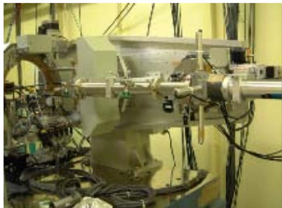
*Fig. 1. Diffractometer at BL16XU used for the reflectivity measurement. Vacuum pipes are placed at upstream of the sample and between the sample and the detector to prevent absorption of X-rays in air.*
