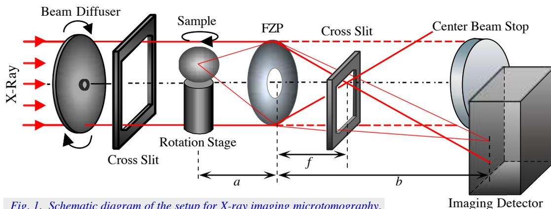
Fig. 1. Schematic diagram of the setup for X-ray imaging microtomography.  $a = 176 \text{ mm}$  and  $b = 1760 \text{ mm}$  (magnification is  $\times 10$ ),  $f = 160 \text{ mm}$ .
