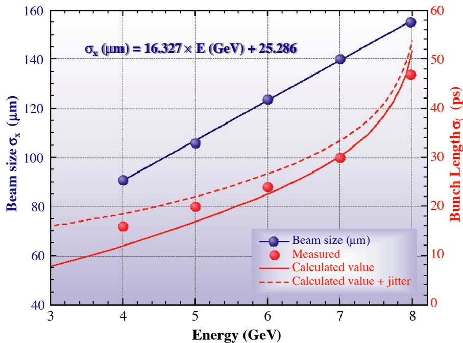
Fig. 5. Horizontal beam size and bunch length as a function of beam energy.
