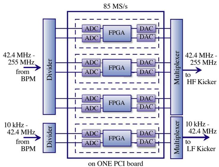
Fig. 4. Block diagram of a digital signal-processing unit with four modules on one PCI board.
