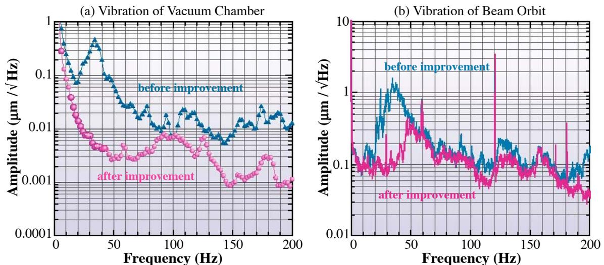
Fig. 1. Vertical vibration of the vacuum chamber and the stored electron beam before and after improvements.
