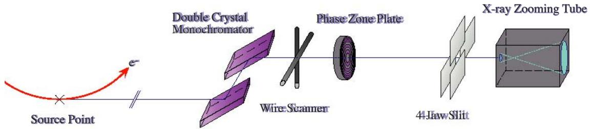
Fig. 3. Optical system of the X-ray imaging of the electron beam.
