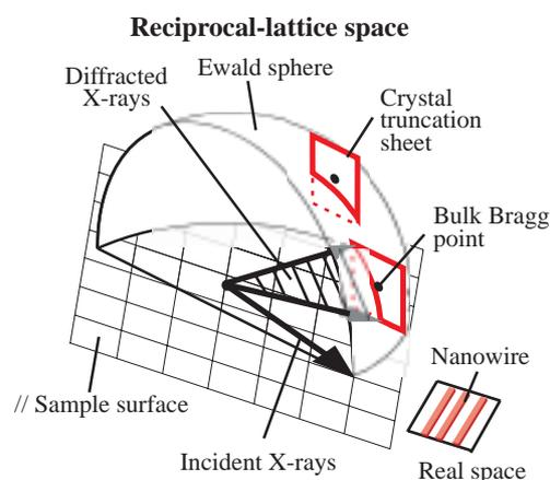
Fig. 2. Geometry of grazing-angle high-energy X-ray scattering.
