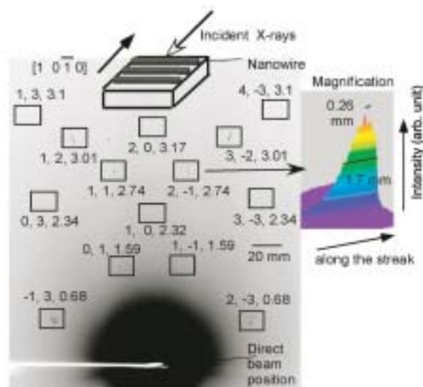
Fig. 3. Pattern diffracted from nanowires nearly perpendicular to the incident X-ray beam. The distance from sample A to the imaging plate (camera length) was 190 mm. A pair of numbers  $h, k$  stands for an index of a crystal truncation sheet. The lengths used for unit vectors  $\mathbf{a}$  (//  $[1\ 0\ \bar{1}\ 0]$ ),  $\mathbf{b}$  (//  $[0\ 1\ \bar{1}\ 0]$ ), and  $\mathbf{c}$  (//  $[0\ 0\ 0\ 1]$ ) were 0.476, 0.476, and 0.421 nm, respectively.
