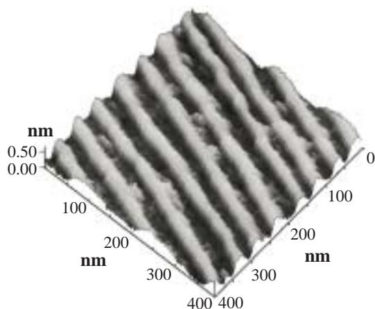
Fig. 1. AFM image ( $0.4\ \mu\text{m} \times 0.4\ \mu\text{m}$ ) of the nanowires grown on an ultrasmooth sapphire surface of sample A.
