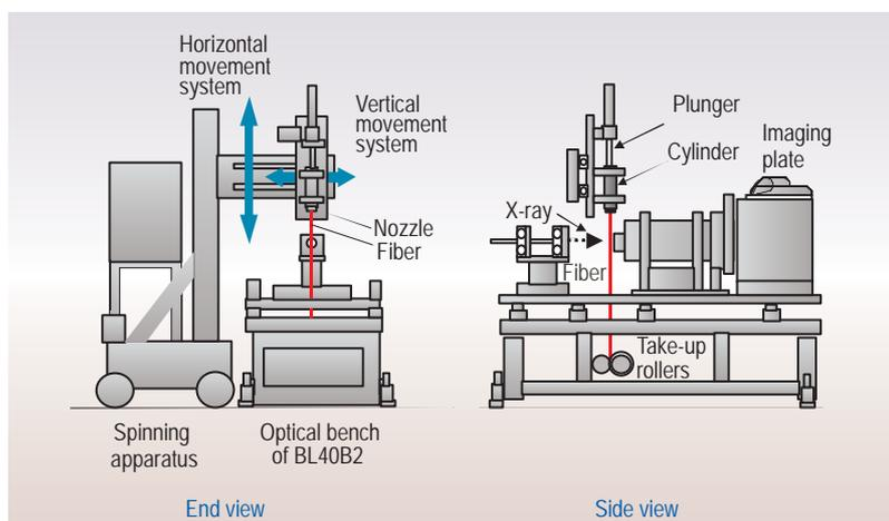
Fig. 1. Schematic representation of the spinning apparatus for *in situ* small-angle X-ray scattering in BL40B2.
