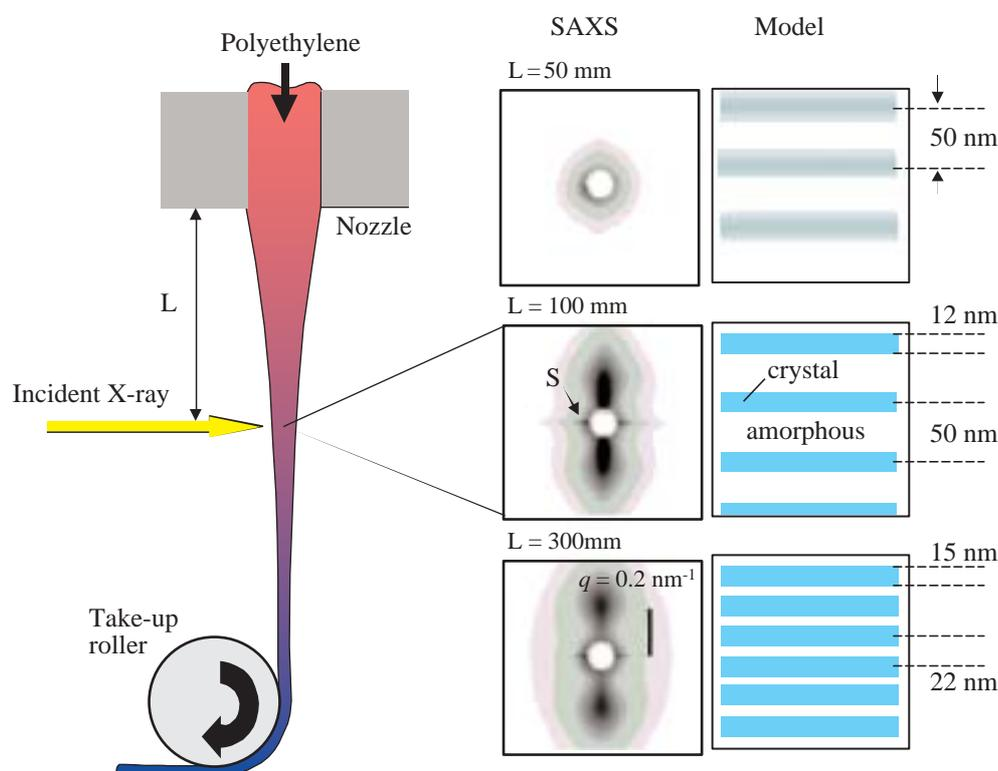
Fig. 2. *In situ* SAXS patterns obtained in the spinline.  $L$  is the distance from the nozzle to the incident X-ray beam. SAXS patterns inserted in this figure are taken at  $L = 50, 100$  and 300 mm. A structure model derived from the analysis of the  $q$  dependence of scattered intensity parallel to the fiber is depicted on the right side of each SAXS pattern.
