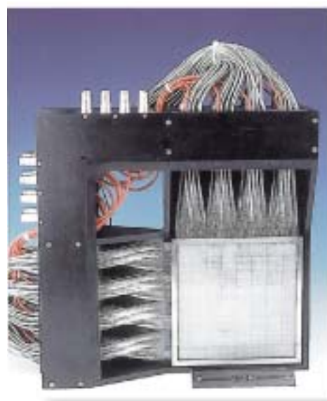
Fig. 2. Photograph of YAP Imager fabricated at the SPring-8 facility.
