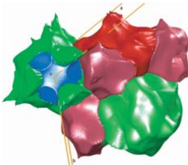
Fig. 3. Atomic surfaces defined by the Bader zero flux condition. The Zn 4 Sb 3 structure is viewed nearly along the c -axis. The light shiny green basins along the c -axis correspond to the “dimer” Sb atom. At the top of the Sb dimer a non nuclear maxima (blue) fits exactly into the void. The red basin is the main Zn atom, the purple basins the interstitial Zn atoms, and the matt green basin is the Sb 3- ion.
