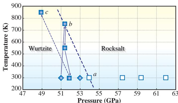
Fig. 4. Results of synthesis experiments on GaN. Solid diamond: wurzite-type; solid square: rocksalt-type; open square: composite of wurzite- and rocksalt-types.
