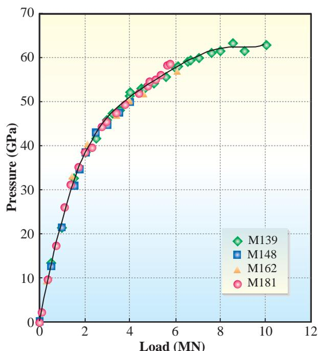
**Fig. 2.** Pressure versus press load at 300 K. Pressure values are based on the MgO scale.
