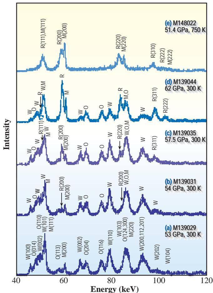
Fig. 3. Selected diffraction profiles of GaN sample with indices. W: wurzite-type GaN; R: rocksalt-type GaN; M: MgO; O: Ga<sub>2</sub>O<sub>3</sub>.
