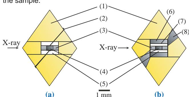
**Fig. 1.** Cross sections of the specimen assemblies employed in experiments at 300 K (a) and at high temperatures (b). (1): Pressure medium; (2): Pt wire; (3): Diamond powder; (4): GaN sample; (5): MgO capsule; (6): LaCrO<sub>3</sub>; (7): Nichrome heater; (8): TiC electrode.
