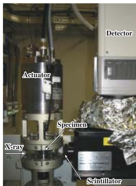
Fig. 2. The test rig specially designed for tomographic in situ observations in the experimental hutch.
