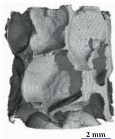
Fig. 1. Tomographic image of typical aluminium foam.
