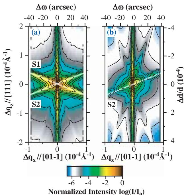
Fig. 3. Reciprocal space maps of samples 1 (a) and 2 (b) within the [111]-[01-1] plane around the 111 reciprocal space point.
