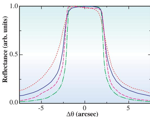
Fig. 1. Rocking curves of the 111 reflection in the reflection geometry for samples 1 (dotted line) and 2 (solid line) measured on the entire surface, sample 2 with a beam size of  $0.5 \times 0.5 \text{ mm}^2$  (broken line), and the theoretical curve calculated using the DuMond diagram (dot-dashed line).
