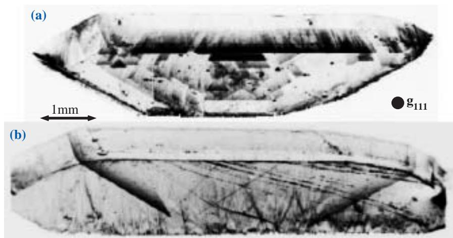
Fig. 2. Reflection topographs with the 111 reflection of samples 1 (a) and 2 (b) measured at the lower tail of the rocking curve.
