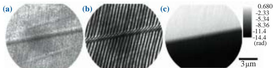
Fig. 3. X-ray micrographs of  $75\text{-}\mu\text{m}$ -thick Kapton film: (a) Absorption-contrast image. Only the sample edge is slightly observed. (b) Interference pattern. The fringe dislocations at the sample edge are clearly observed. (c) Retrieved phase-shift image. The sample is observed clearly and the absolute phase shift is evaluated to be  $12.0\ \text{rad}$ .
