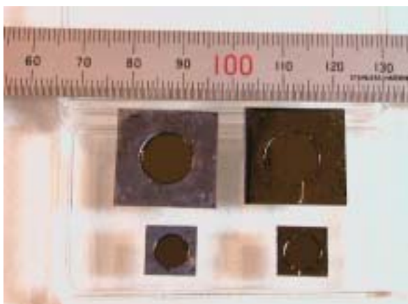
Fig. 2. Transmitting-type Sc/Cr multilayers fabricated by X-ray Co., Ltd. [3]. The front and back surfaces of the phase shifters are shown. The central part transmits light where there is no substrate.
