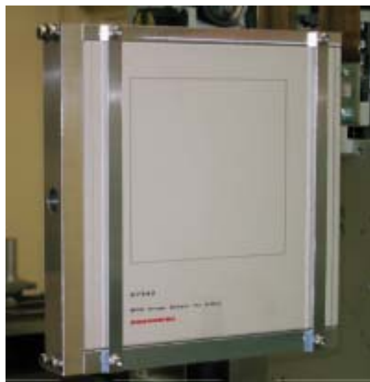
Fig. 1. Photograph of flat-panel detector. The frame drawn in black is the detection area, which has an area of 112 mm × 117 mm.
