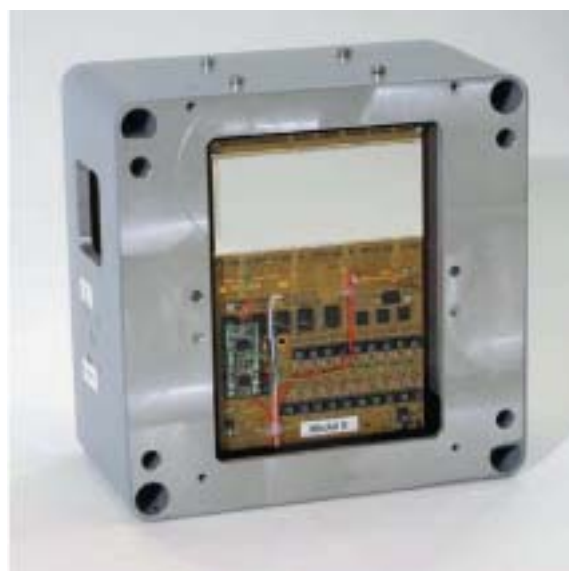
Fig. 1. A single-module pixel detector with 366 \times 157 pixels.
