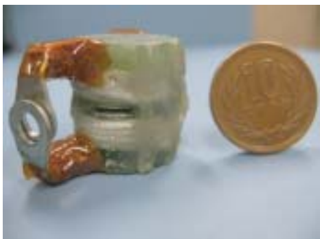
Fig. 1. Photograph of miniature split-pair type magnet for X-ray diffraction.
