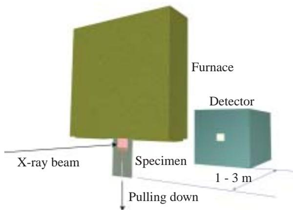
**Fig. 1.** Configuration of specimen, furnace and X-ray detector for observing solidification of Sn-Bi alloys and Al-Cu alloys.
