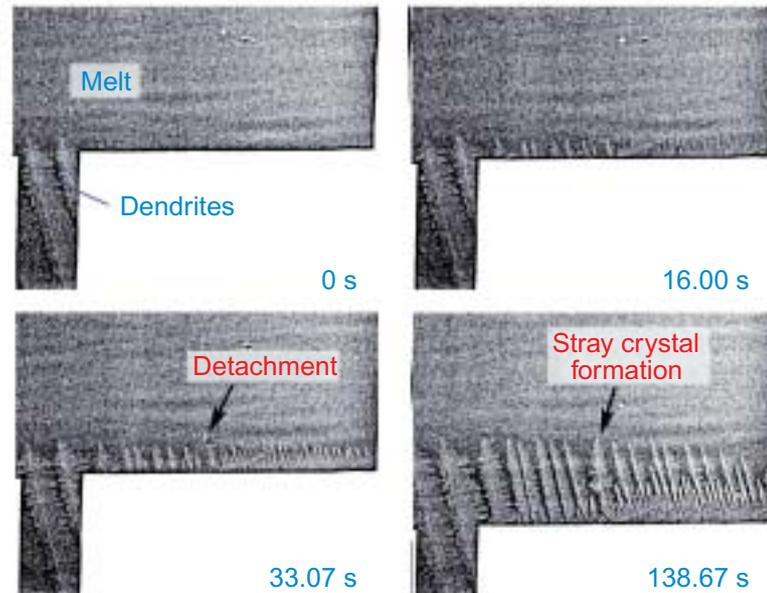
Fig. 2. Sequential photographs of microstructure after dendrites pass re-entrant corner during unidirectional solidification of Sn-21mass%Bi alloy at growth rate of 10  $\mu\text{m/s}$ . The X-ray energy was 29 keV, which is just below the Sn edge.
