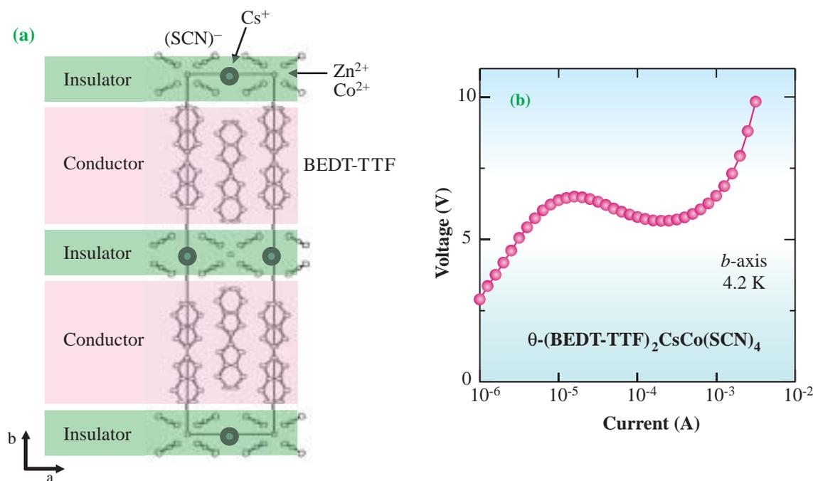
Fig. 1. (a) Crystal structure of  $\theta\text{-(BEDT-TTF)}_2\text{CsM(SCN)}_4$  ( $\text{M}=\text{Co}$  and  $\text{Zn}$ ). (b) Voltage-current characteristics for  $\text{M}=\text{Co}$  at 4.2 K. The current was applied along the  $b$ -axis direction.
