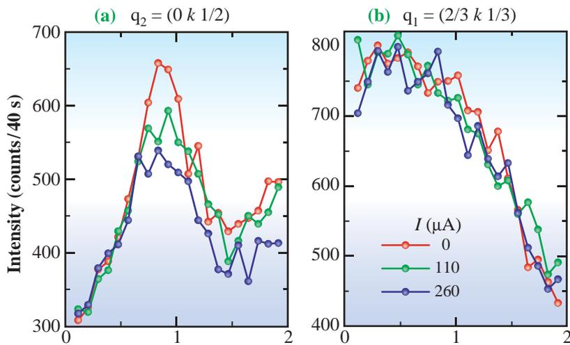
Fig. 2. Diffuse peaks for competing charge ordered domains for various external currents. (a)  $q_2 = (0 k 1/2)$  and (b)  $q_1 = (2/3 k 1/3)$ . Only the  $q_2$  peak loses its intensity with increasing current.
