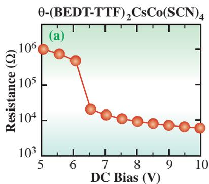
Fig. 3. DC-to-AC conversion in  $\theta$ -(BEDT-TTF)<sub>2</sub>CsM(SCN)<sub>4</sub>. (a) Nonlinear resistance as function of DC bias voltage. (b) AC component of current flowing through sample. (c) FFT spectra for (b).
