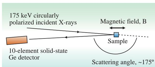
Fig. 1. A schematic of the experimental configuration used to measure spin-polarized Compton profiles on BL08W.
