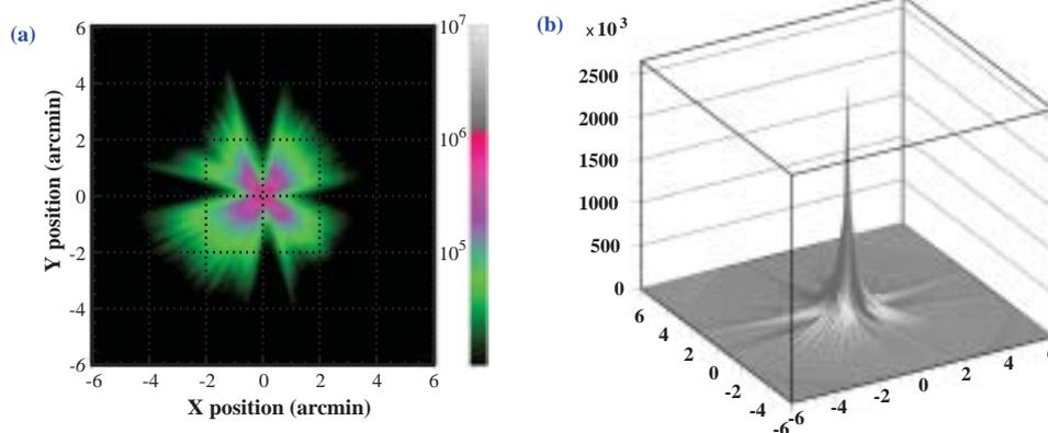
Fig. 2. Focused image of hard X-ray telescope at 30 keV. (a) Two-dimensional expression with color coding in log scale. (b) Three-dimensional expression. Horizontal axes are in arcmin.
