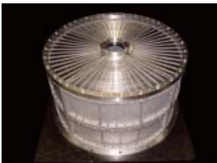
Fig. 1. Multilayer supermirror hard X-ray telescope.
