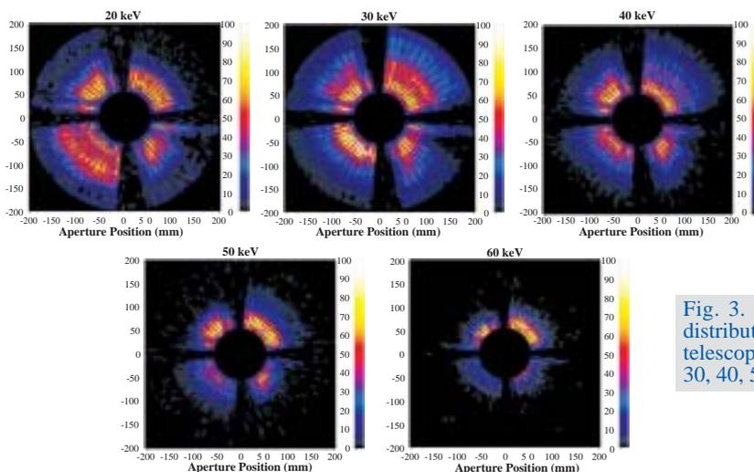
Fig. 3. Local brightness distribution of hard X-ray telescope measured at 20, 30, 40, 50 and 60 keV.
