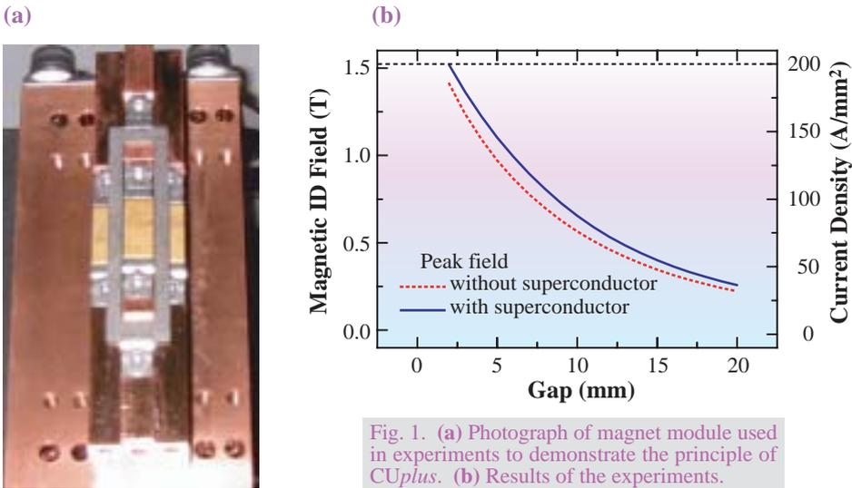
Fig. 1. (a) Photograph of magnet module used in experiments to demonstrate the principle of *CUplus*. (b) Results of the experiments.
