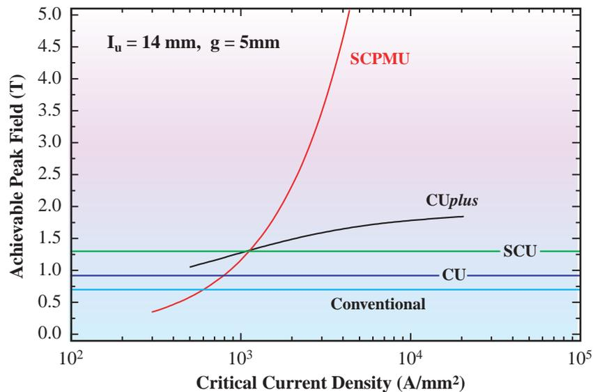
Fig. 4. Expected performance of proposed undulator and comparison with that of existing undulators.
