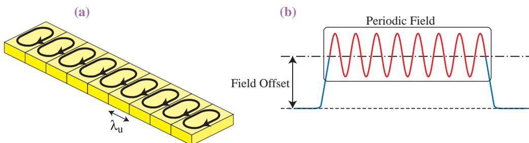
Fig. 2. (a) SCPM array with identical polarity and (b) its typical field profile.
