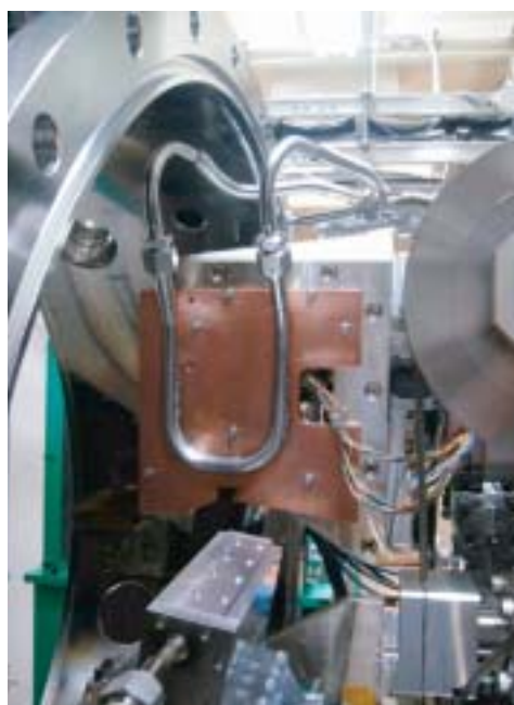
Fig. 2. Compton shield (KOHZU Precision Co., Ltd.) installed to second cradle.
