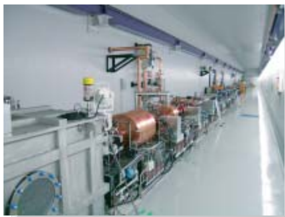
Fig. 4. SCSS test accelerator, prototype of X-ray FEL. Construction was completed in November 2005. First lasing test at 60 nm wavelength is scheduled in June 2006.
