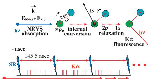
Fig. 2. Schematic illustration of the NRVS measurement. Left to right: monochromatic photons from SPring-8 beamline BL09XU excite an  $^{57}Fe$  nucleus and a vibration with frequency  $\omega$ . The excited  $^{57}Fe$  nucleus relaxes by internal conversion with a lifetime of ~100 ns by expelling a  $1s$  electron. The subsequent  $K\alpha$  radiation is measured between synchrotron pulses (bottom) by an avalanche photodiode detector.
