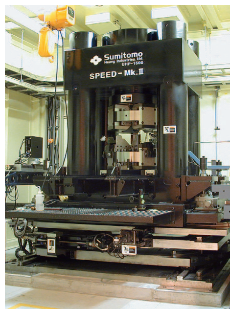
Fig. 1. Kawai-type apparatus called "SPEED-Mk.II", which is installed at BL04B1.
