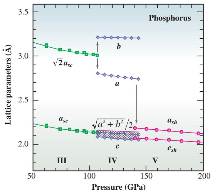
Fig. 3. Pressure dependence of the lattice parameters for phosphorus phases III, IV, and V. The squares, diamonds, and circles denote the lattice parameters for each phase. The crosses correspond to the nearest distance in the  $ab$  plane in phase IV. The pink-hatched area above the  $c$  axis length shows the nearest distance along the  $c$  axis, which is elongated by the modulation.
