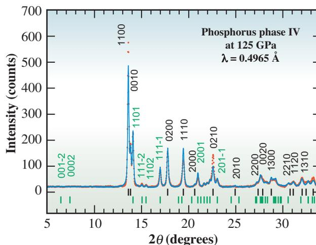
Fig. 2. Diffraction pattern of phosphorus phase IV observed at 125 GPa (brown dots) and the Rietveld fit with the proposed  $Cmmm(00\gamma)s00$  model (blue curve). The upper and lower tick marks show the peak positions of the fundamental and satellite reflections, respectively.
