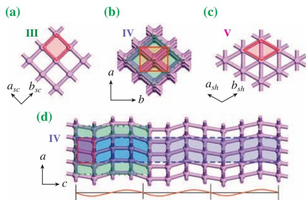
Fig. 1. Crystal structures of phosphorus (a) phase III, (b) phase IV, (c) phase V in  $ab$  plane, and (d) phase IV in  $ac$  plane with a commensurate approximation. The dashed blue rectangle in (d) represents the 11 times supercell. The solid red rectangles in (b) and (d) show the fundamental lattice for the  $Cmmm(00\gamma)s00$  model. The dotted green rectangle in (d) shows a monoclinic lattice predicted by Ishikawa *et al.* [2].
