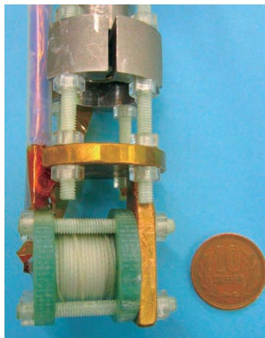
**Fig. 1.** Photograph of the solenoid-type miniature magnet used for the X-ray absorption measurement.
