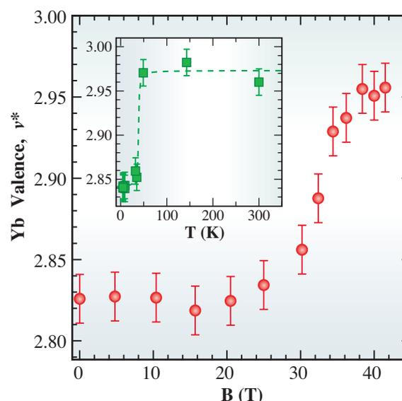
Fig. 3. Magnetic field dependence of the valence at 5 K. The inset shows the temperature dependence of the valence at zero magnetic field.
