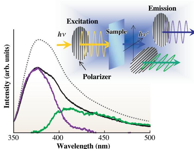
Fig. 2. Fluorescence (dotted line) and the polarized fluorescence spectra of melem in the PrSA film ( $\lambda_{\text{ex}} = 280 \text{ nm}$ ) with the vertical or the horizontal emission polarizer, which can be resolved into two components (blue and green).
