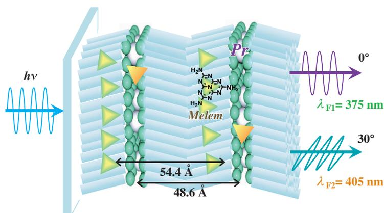
Fig. 3. Illustration of dual polarized emissions of melem arranged in the PrSA film.
