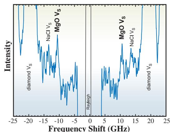
Fig. 4. Brillouin spectrum of polycrystalline MgO at 49 GPa and  $\sim 2300 \text{ K}$ .
