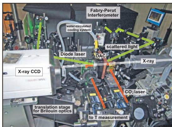
Fig. 2. View of the whole Brillouin scattering measurement system combined with synchrotron X-ray diffraction and laser heating systems at BL10XU. Green, white and red lines indicate the schematic optical paths for Brillouin scattering measurement, X-ray diffraction measurement and the laser heating system, respectively.
