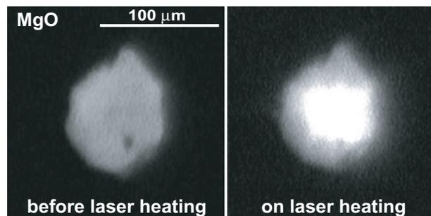
Fig. 3. Photomicrographs of polycrystalline MgO in a DAC before laser heating (at 45 GPa) and during laser heating (at  $\sim 2300 \text{ K}$ ).
