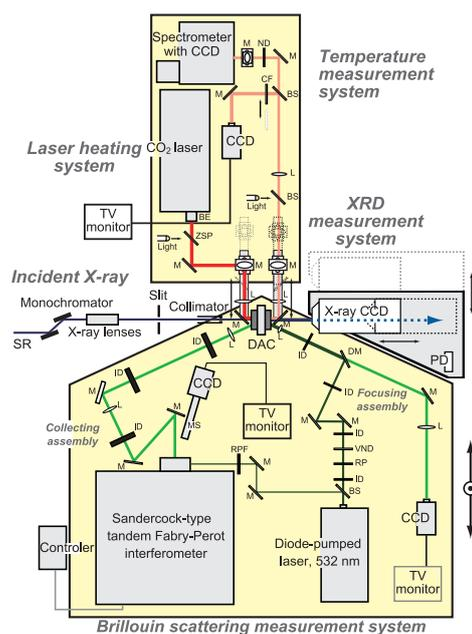
Fig. 1. Schematic layout of the Brillouin scattering measurement system combined with synchrotron radiation and infrared laser heating system of BL10XU beamline.
