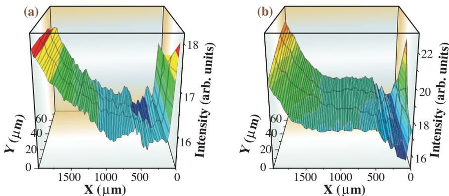
Fig. 4. Mapping images of the -OH functional group of the chromane ring in vitamin E. The X axis is along the depth direction and the Y axis is along the surface of the artificial joint. (a) After accelerated oxidation and knee simulator. (b) Before accelerated oxidation and knee simulator (control).
