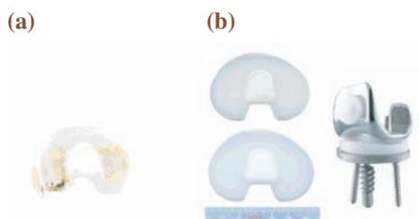
Fig. 1. (a) Failed UHMWPE knee component due to lack of oxidation stability. (b) Test sample (top), control (bottom) and HTK II knee joint.
