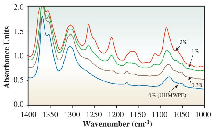
Fig. 3. Infrared absorption spectra of UHMWPE with various concentrations of added vitamin E.
