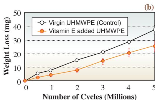
Fig. 2. (a) AMTI knee joint simulator. (b) Weight loss of the samples during the simulation.
