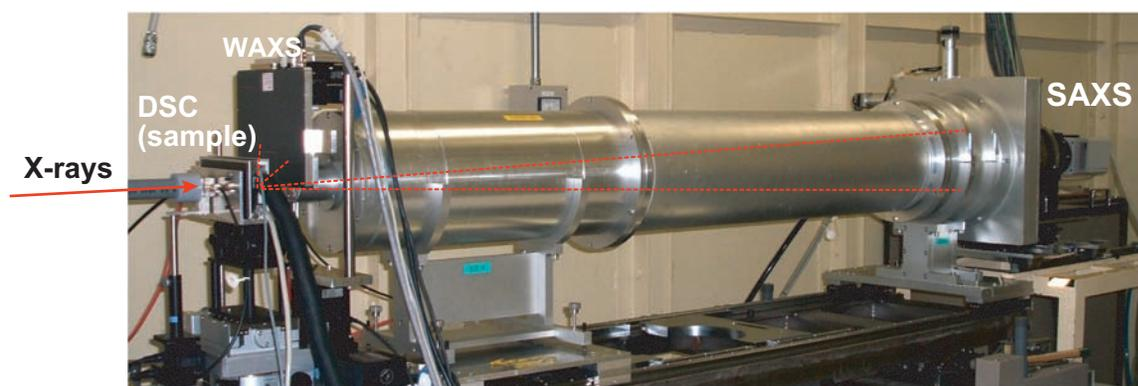
Fig. 1. Photograph of the DSC/WAXD/SAXS simultaneous measurement system built-up at beamline BL40B2.
