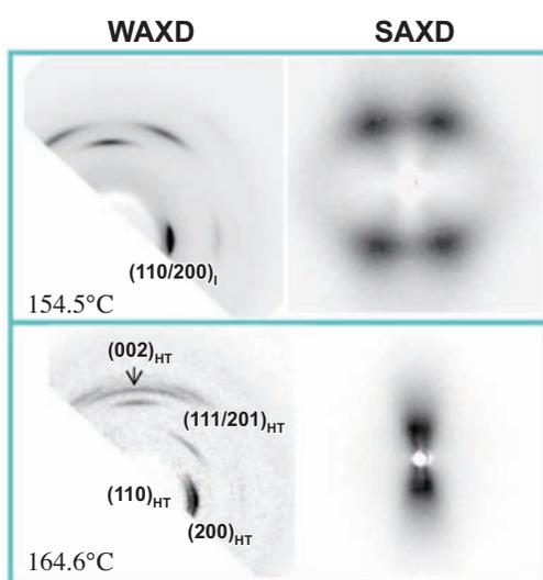
Fig. 2. WAXD and SAXS patterns measured simultaneously for oriented PVDF sample at 154.5 °C and 164.5 °C. The meridional direction is parallel to the oriented direction of sample.
