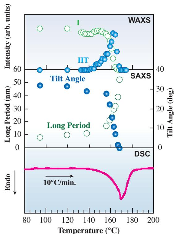
Fig. 3. Temperature dependences of long period and tilting angle of stacked lamellae, peak intensity of the (001)I and (002)HT reflections and DSC thermogram measured for the uniaxially-oriented PVDF form I in the heating process at 10.0 °C/min.
