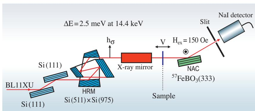
Fig. 1. Optics for the energy domain SR Mössbauer spectroscopy using single-line pure nuclear Bragg scattering. (HRM: high-energy-resolution monochromator; NAC: nuclear analyzer crystal).
