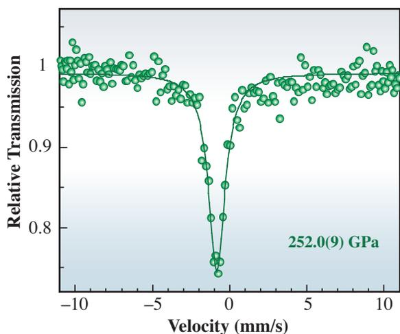
Fig. 3. SR Mössbauer spectrum of a polycrystalline iron metal ( $^{57}\text{Fe}$  95%) in DAC at ultrahigh pressure of 252 GPa. The solid line is fit with Lorentzian line.
