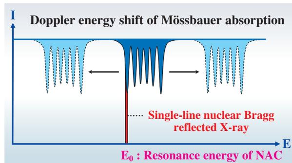
Fig. 2. Conceptual diagram for the energy domain SR Mössbauer spectroscopy with single-line pure nuclear Bragg scattering.
