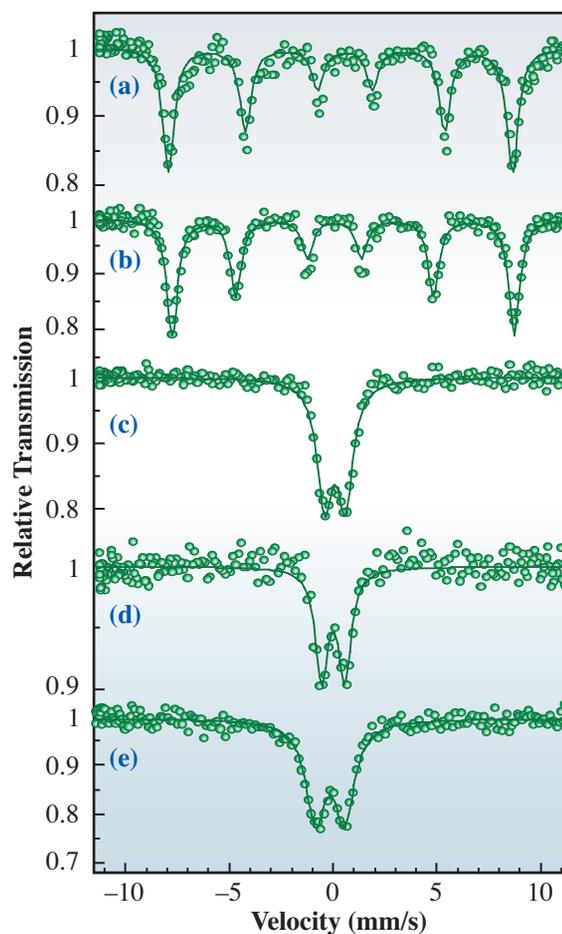
Fig. 4. SR Mössbauer spectra of  $^{57}\text{Fe}_2\text{O}_3$  at different pressure conditions. (a) 0 GPa, (b) 43 GPa, (c) 91 GPa, (d) 121 GPa and (e) 204 GPa. The solid lines are fits with Lorentzian lines.
