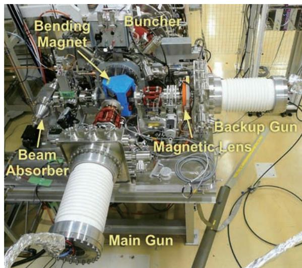
Fig. 25. Twin electron gun.
