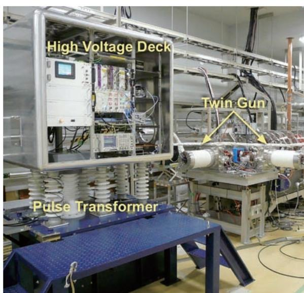
Fig. 24. New high-voltage station installed in the accelerator room.
